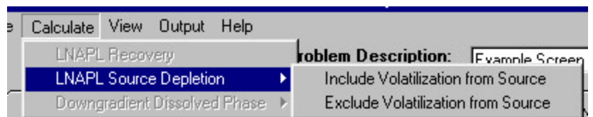
Figure 5-21. The source depletion calculation options, with or without volatilization from the LNAPL source.
